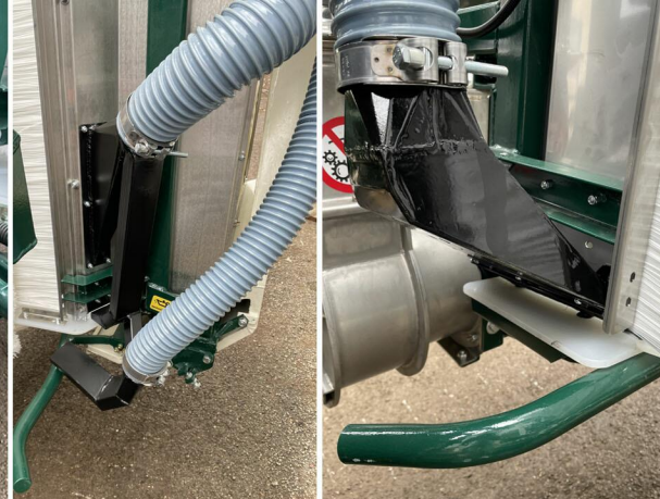
SISTEMA A FLUSSI D'ARIA MULTIPLI SYSTEM WITH MULTIPLE-AIR JET DEFLECTOR
